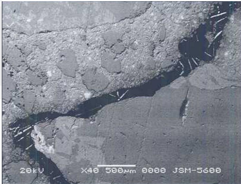
Crystals have formed in the crack
