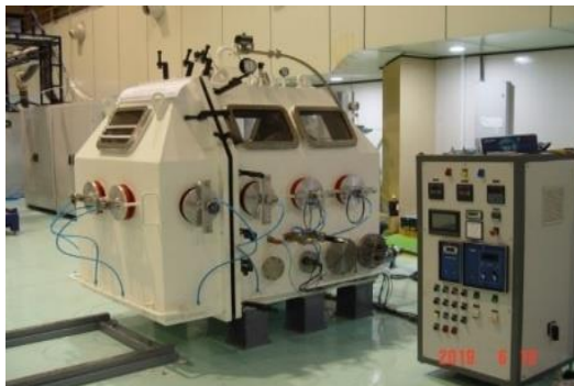
Welding Glove-box for Cavity Dressing
