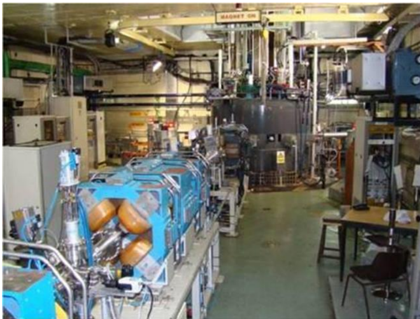
Fig. 4.1.5: Photograph of K500 superconducting cyclotron built at VECC, Kolkata
