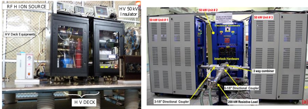
Fig. 4.4.1: RF discharge based H- ion source (left) and 325 MHz, 150 kW Solid State Amplifier (right) developed at RRCAT.
