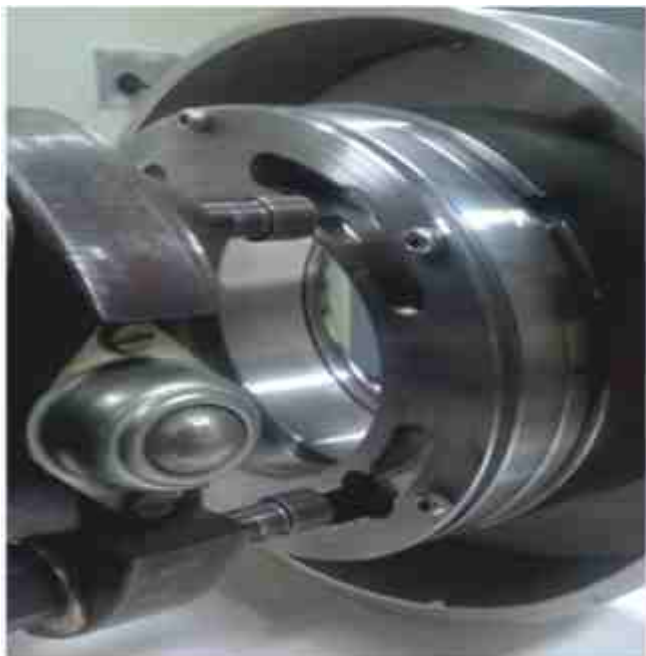
Helium leak tight Remotely Operated Self-Locking Fixture
