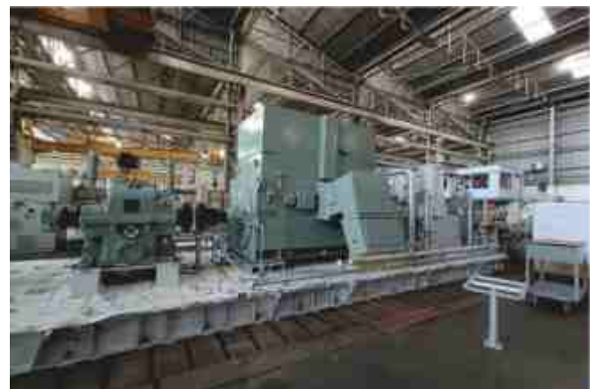
Indigenously Developed BFP at Vendor's Workshop
