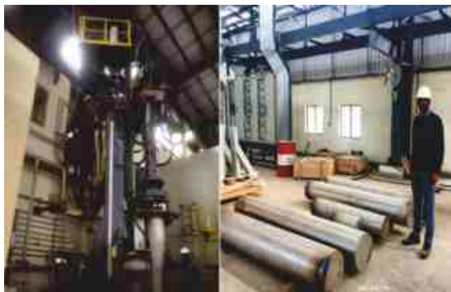
Vacuum Arc Remelting furnace with trial melts
