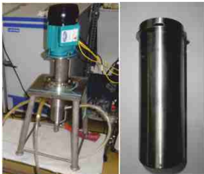
Photographic view of single stage ACE 60 mm setup (a) Complete ACE setup with drive and (b) 60 mm ID ACE rotating bowl
