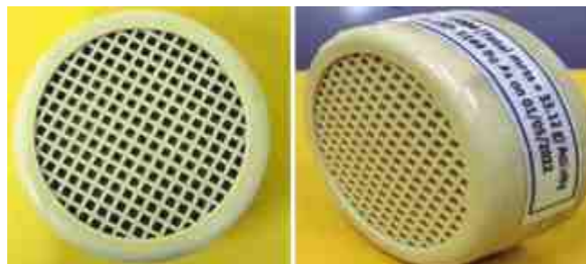
Charcoal cartridge standards for calibration of Iodine monitors
