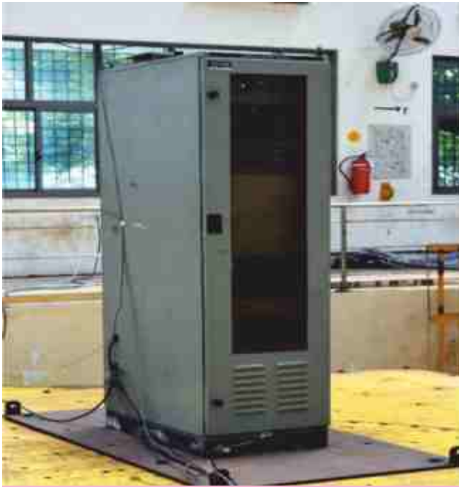
Cabinet mounted on Shake Table
