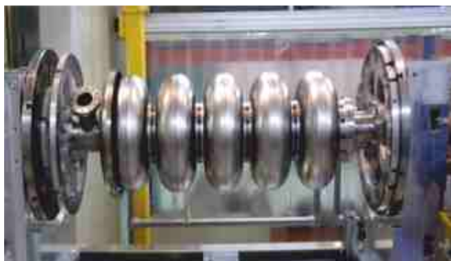
Elliptically shaped 5-cell 650 MHz SCRF bare cavity
