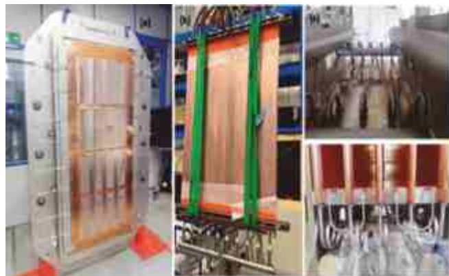
DNB components a) grids of beam source, b) RID panel c) neutralizer under assembly
