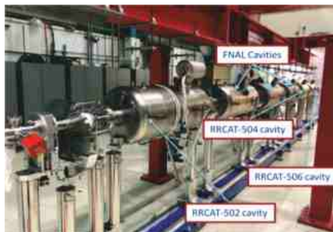
String Assembly for pCM of PIP-II with 3 cavities from RRCAT, India and 3 from Fermi lab, USA
