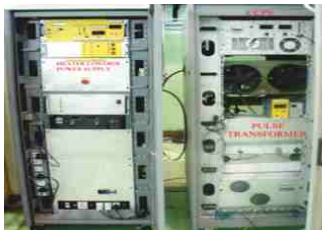
90 kV solid state pulse modulator assembly
