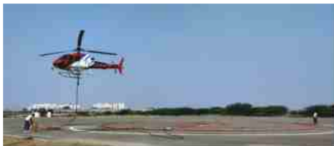
Preparation of heliborne geophysical survey with VTEM system, Rajasthan
