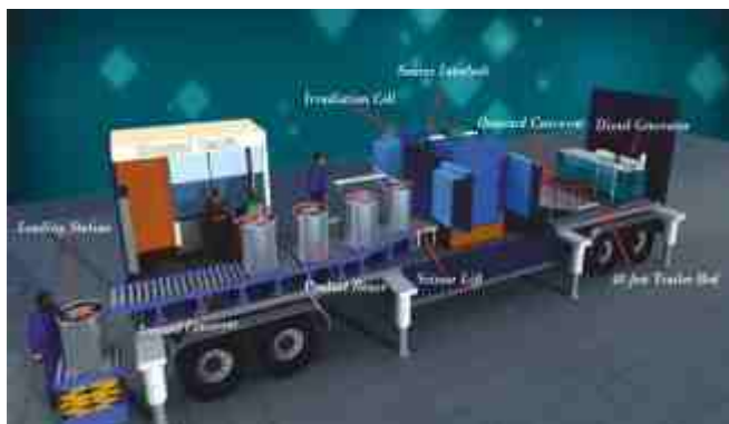
Schematic layout of Mobile Food Irradiator
