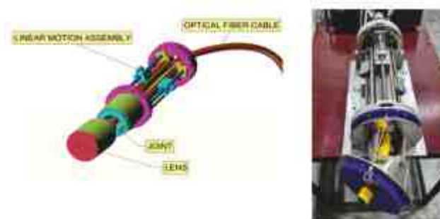
Prototype manipulator for maneuvering the lens bundle
