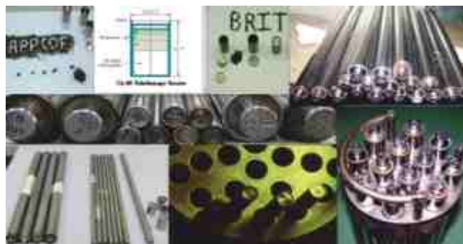
High intensity Cobalt-60 Sealed sources (Cobalt-60 Teletherapy Sources (CTS), W-91 and BC-188 irradiator sources) fabricated at RAPPCOF
