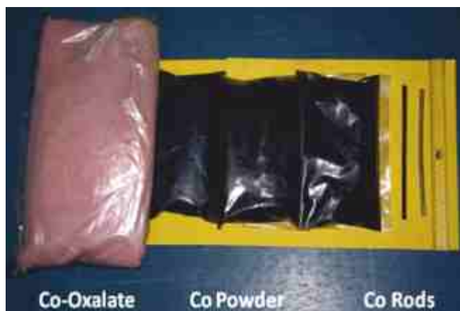
Cobalt and associated materials recovered from maraging steel scrap
