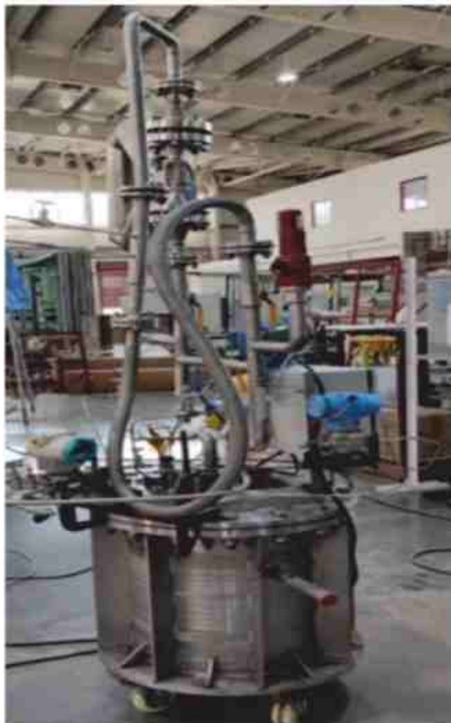
Indigenously developed high pressure helium circulator
