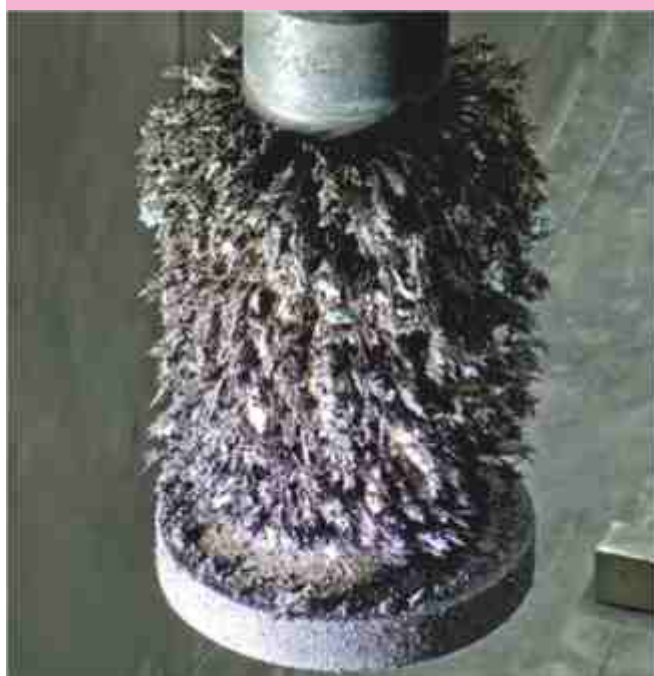
Cathode with 4.5 Kg U deposit
