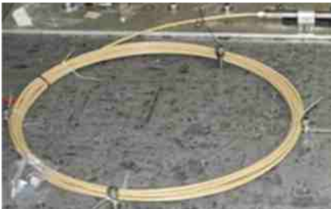
High sensitivity Helium-3 proportional counter for fuel loading in LWR
