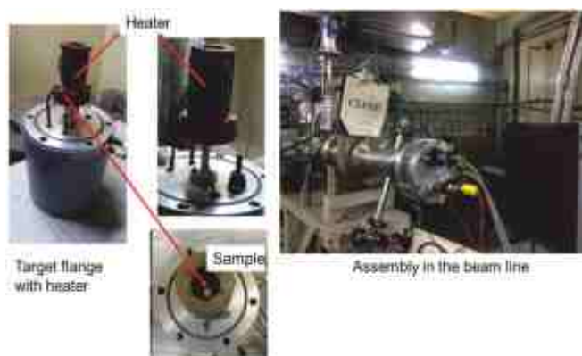
Target flange and its assembly in the beam line at the Cave-1 of the K-130 Cyclotron
