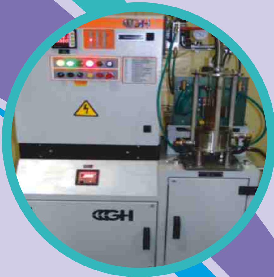
Induction Levitation Melter developed by Bhabha Atomic Research Centre
