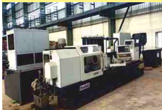
Deep hole drilling machine- Commissioned
