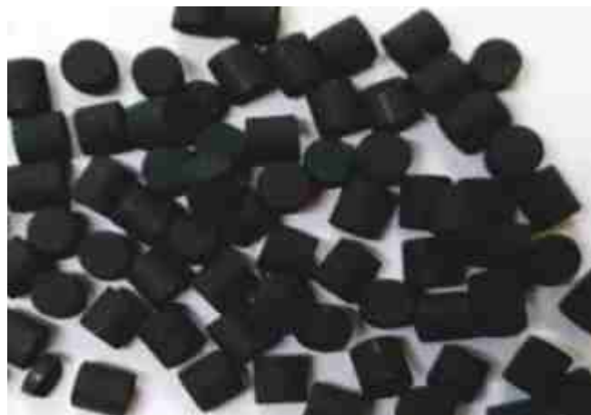
Oxidized Sud Chemie Catalyst
