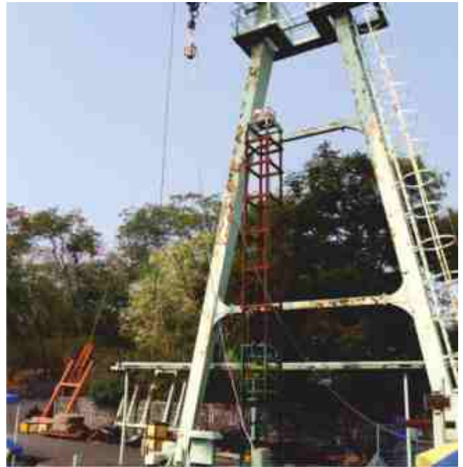
ROTEX-I device hanged at a height of 9m for the drop test
