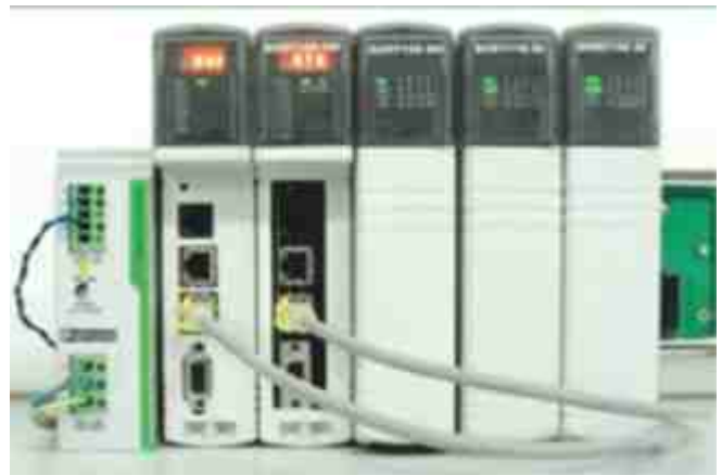
Remote Terminal Unit (RTU)
