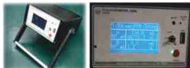
Dual channel Faraday cup electrometer
