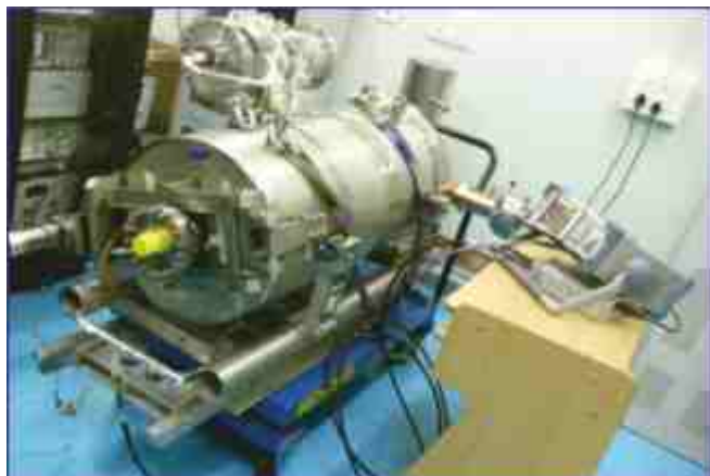
Five cell SCRF cavity with tuner and power Coupler
