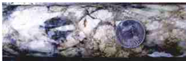
Core of Spodumene bearing pegmatite, Marlagalla, Mandya district, Karnataka
