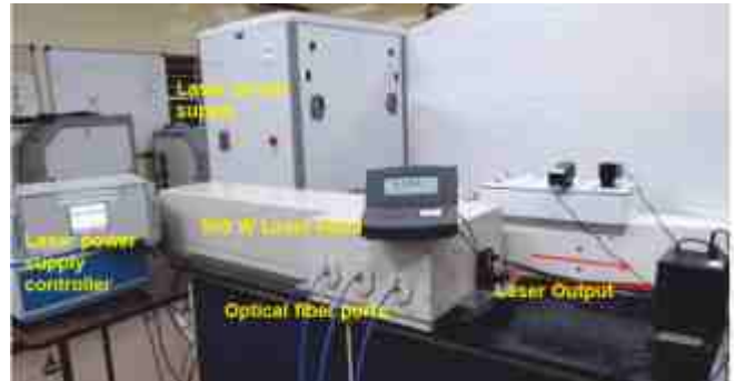
500 W/10 kW Nd: YAG laser for welding application
