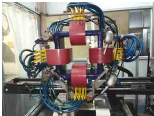
New steering magnet for the Super-conducting cyclotron beam line and measured field profile of the magnet
