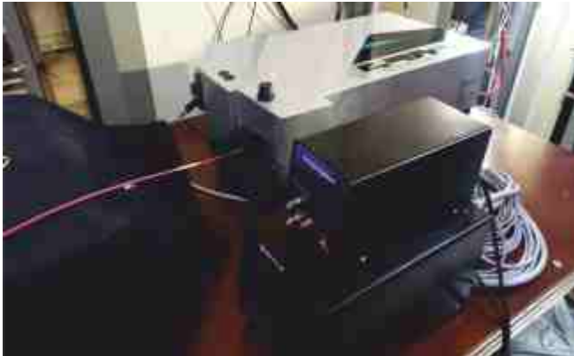
Visible spectrometer developed at IPR for ADITYA-U tokamak
