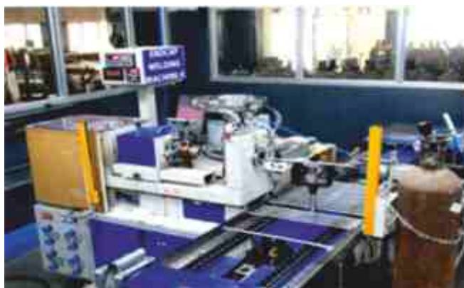
Installation & commissioning of 2 nos. of Automatic end cap welding machines
