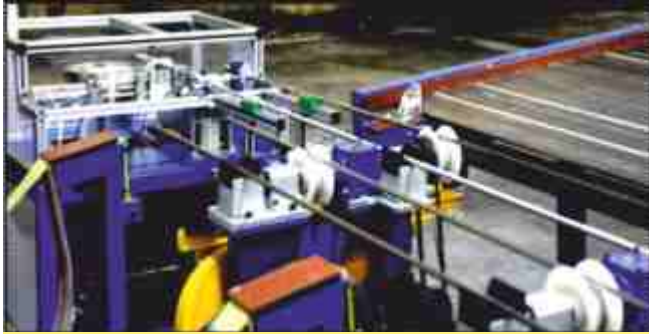
Automatic Tube ID cleaning
