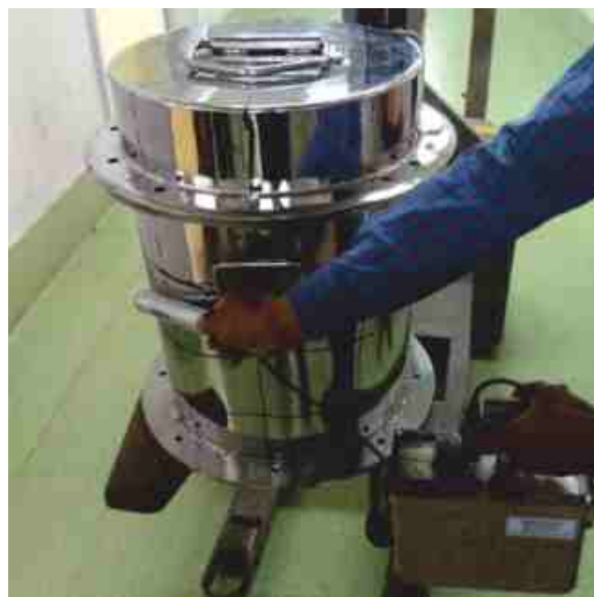
MTP-1200 package during radiometry test
