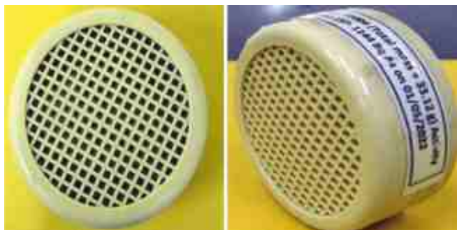
Charcoal cartridge standards for calibration of iodine monitors
