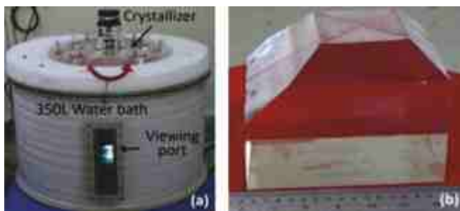
a) Water bath containing 50 L crystallizer; (b) KDP crystal
