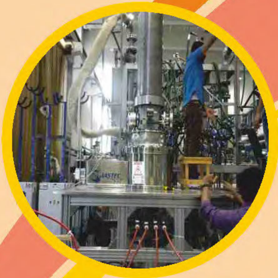
Test Gyrotron at ITER-India lab, IPR
