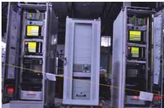
Dhruva ESCADA Panels undergoing burn-in test
