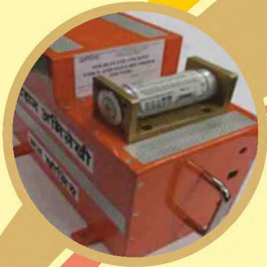
Solid State Cockpit Voice and Data Recorder (SSCVDR) developed by ECIL
