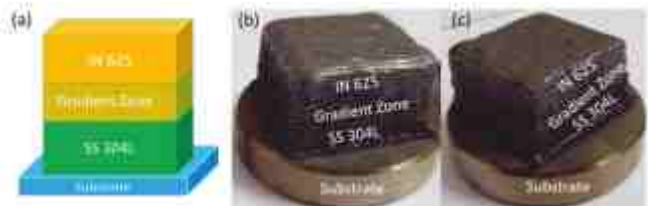
Deposited bimetallic structure of SS304L-IN625 with graded interface
