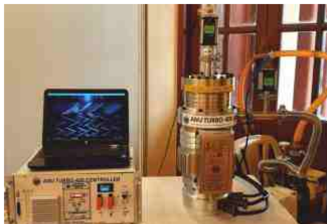
Magnetically suspended Turbo-molecular Pump ANU TURBO-400
