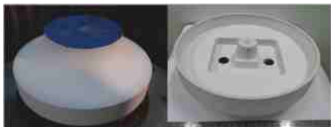
Plasma sprayed alumina coating on solid cathode mounting plate top and bottom view
