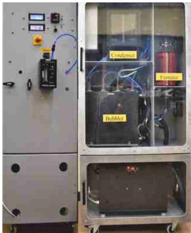
Integrated Tritium and Radiocarbon Sampling System
