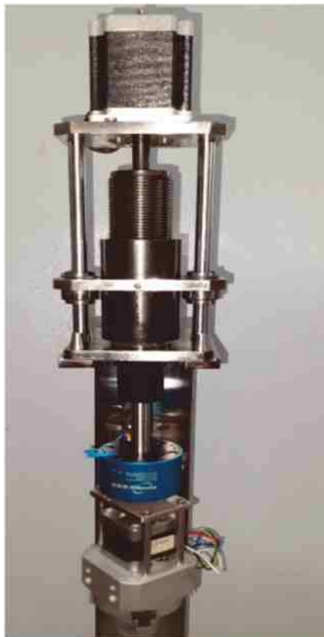
Uni motored Rotary Linear actuator
