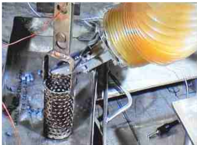
Fuel loaded to anode basket
