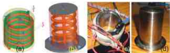
Conformal Cooling Channel- CAD models for (a) external (b) internal and LAM built parts (c) external (d) internal
