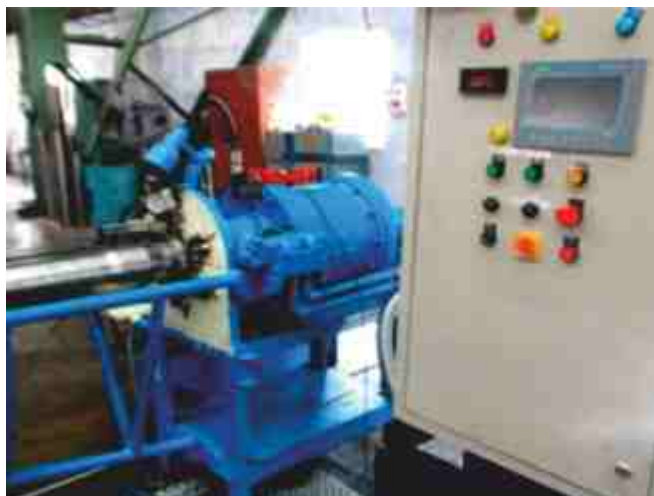
Automation of Calandria tube end flaring machine
