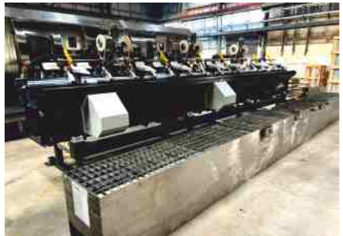
Tube Grinding cum Polishing machine 8-20mm – Received at site
