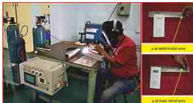
GTA welding of vacuum chamber using Binary Gas Mixing System (BGMS)
