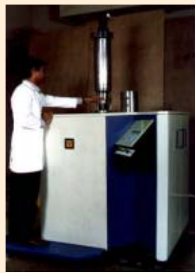
Gamma chamber irradiator developed by BRIT
