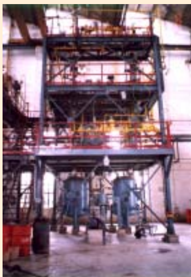
Radiotracer studies on a trickle bed reactor of a factory
