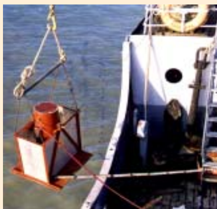
Using radiotracer technique, silt movement is being studied in Hoogly river in West Bengal
