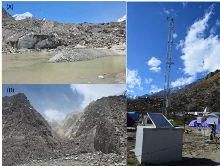
Figure 1. Showing the manual observatory, Automatic Weather Station (AWS), and broadband seismic station established at Bhojwasa.
