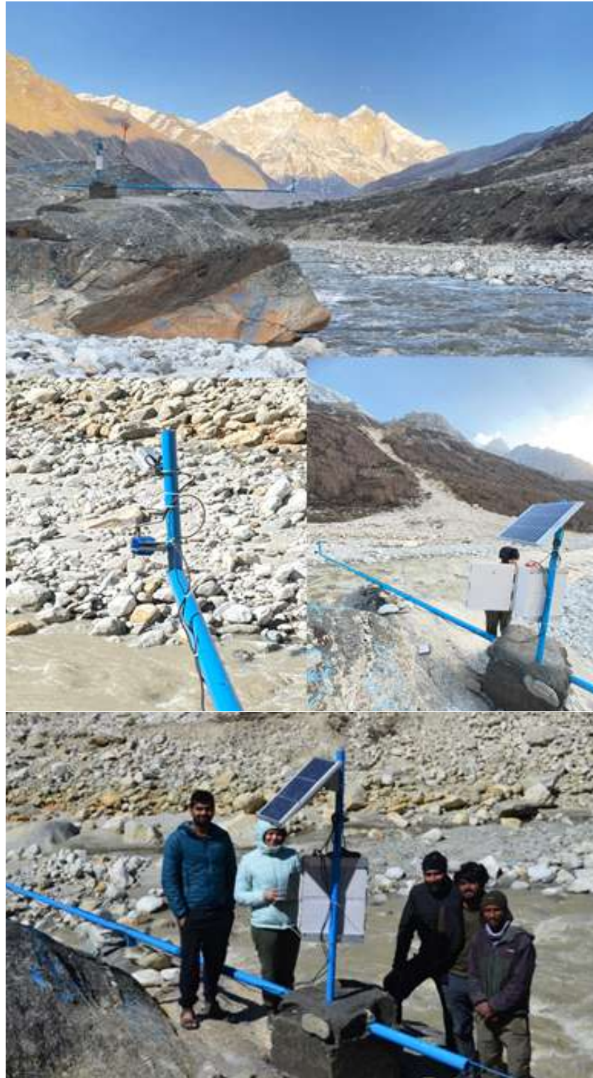
Figure 2. Newly established Automatic Water Level and Velocity Recorder (AWLVR) at the Bhojwasa site, installed for continuous monitoring of stream stage and flow velocity in the Gangotri Glacier meltwater channel.
