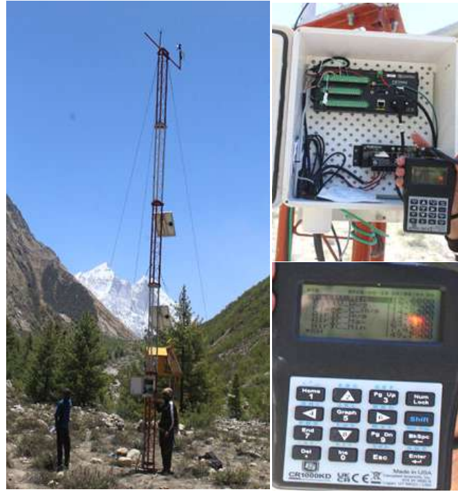
Figure 4. Showing the, Automatic Weather Station (AWS), station established at Chirwasa.
