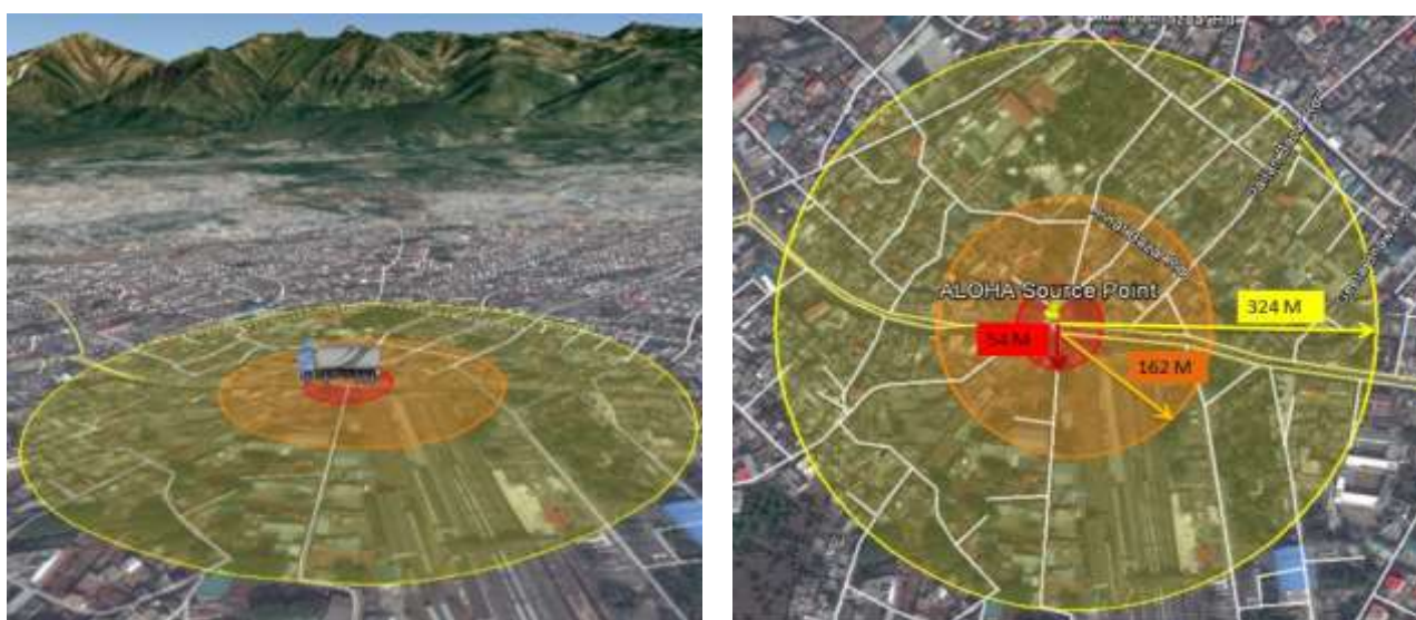
Figure 2.37: Scenario Modelled for a Tanker Explosion During Transport
