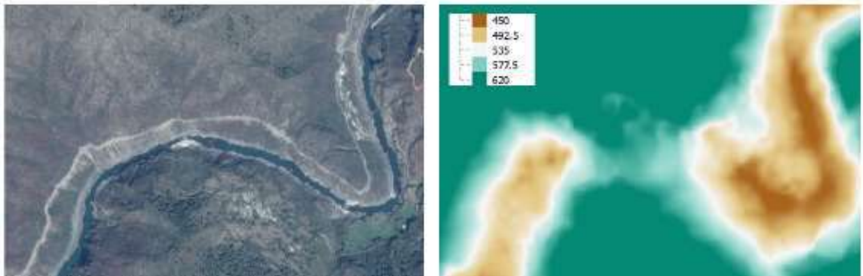
Figure 3.53: Example of inconsistencies and errors frequently encountered in the DEM: Incoherent river elevation profile – river width >80m (steep terrain) not resolved by the 10m DEM product
