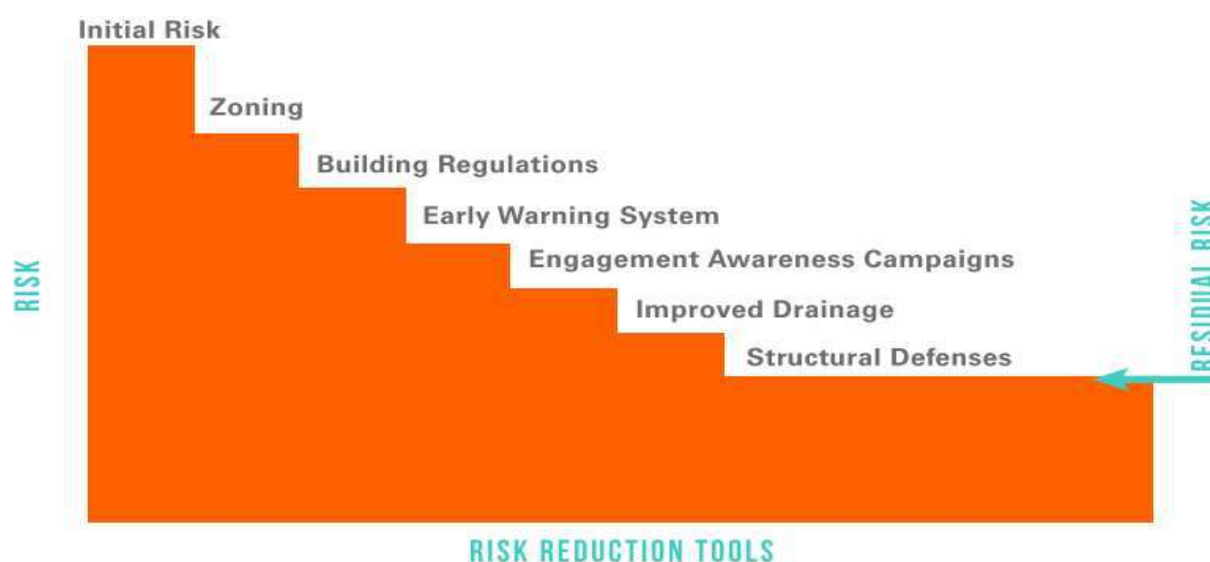
Figure 7.1: “Bringing down the risk” – an illustration of how a selection of mitigation measures progressively reduce flood risk from an initial high to a more acceptable level (moving from left to right) (Source: Verway et al. 2017)
