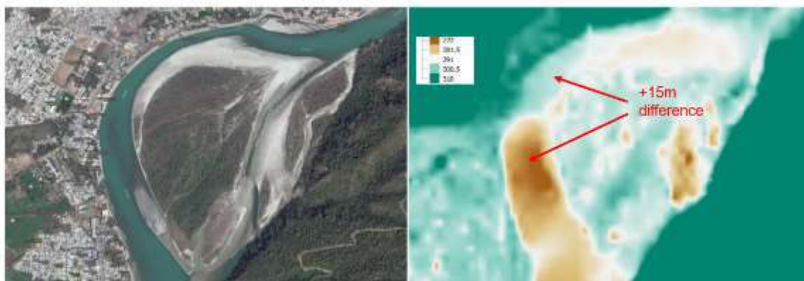
Figure 3.54: Example of inconsistencies and errors frequently encountered in the DEM: Incoherent river elevation profile – river width >200m – flatter terrain
