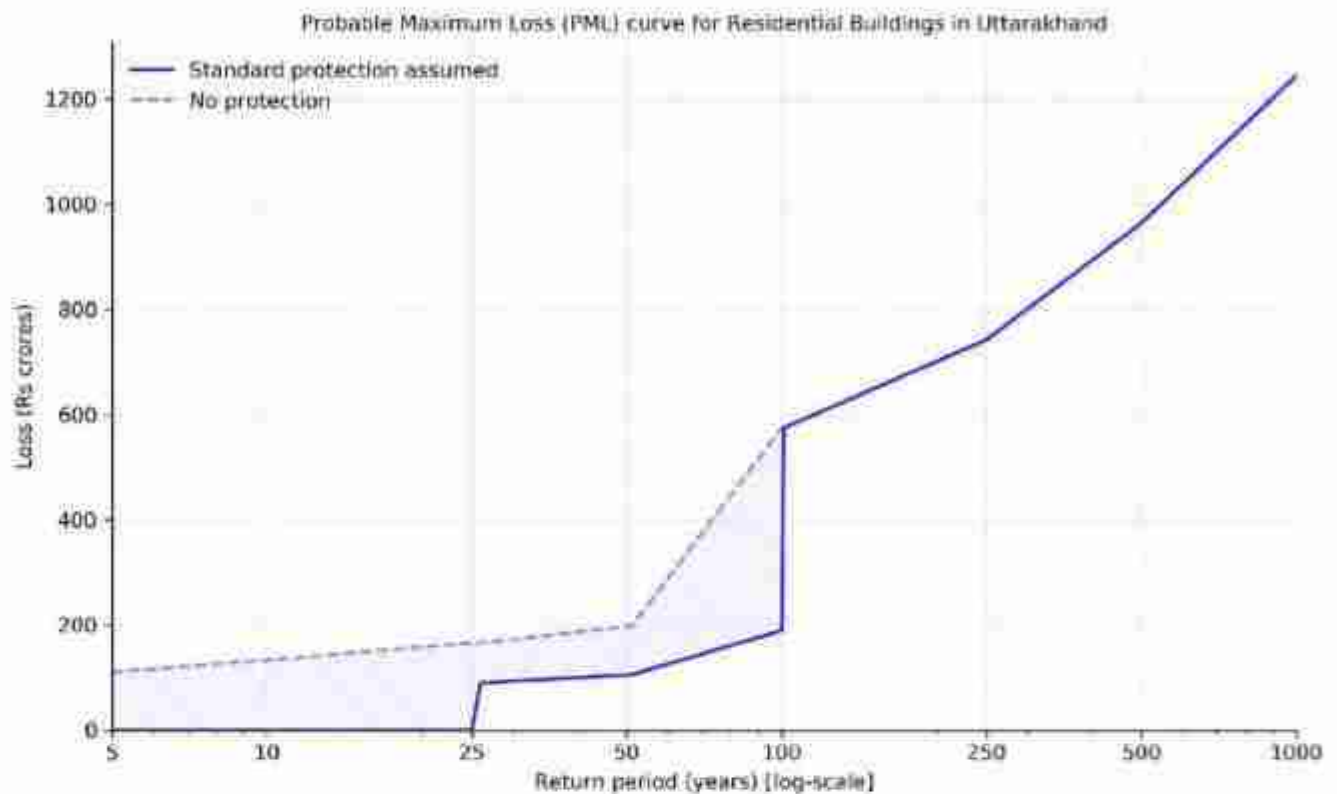
Figure 3.112: Probable Maximum Loss (PML) curve for residential buildings in Uttarakhand due to fluvial floods
