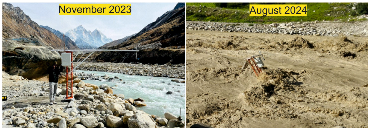
Figure 1: Location of the Automatic Water Level Recorder during the pre-and post-flood events in Bhojwasa.
