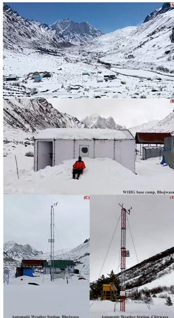
Figure 3. (A) Snow-covered view of Bhojwasa during March 2025; (B) The hut and base camp, fully covered in snow; (C) The observatory at the base camp, equipped with an Automatic Weather Station and Broadband Seismic Station at Bhojwasa; and (D) the Automatic Weather Station at Chirwasa.
