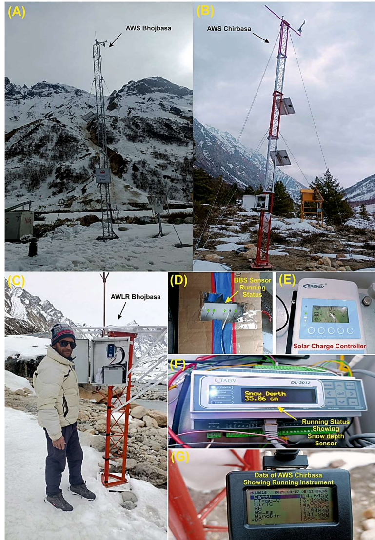
Figure 1. Recent field photos of Installed instruments and the proof, that our instruments are continuously working well and collecting data, (A) AWS at Bhojbasa, (B) AWS at Chirbasa, (C) AWLR at Bhojbasa near Bhagirathi river, (D) data Logger of BBS showing green lights on which means it is continuously working, (E) The charge controller of AWS Bhojbasa, (F) Display of AWS showing snow depth data and other information. (G) The display of data showing AWS at Chirbasa.
