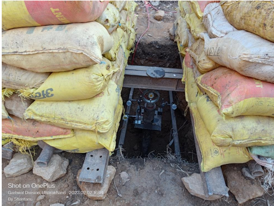
Fig. P3: Plate Load Test at Marwadi (MW) near Jaypee Colony (Ward 2)
