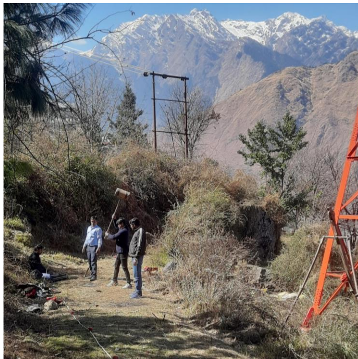
Fig. P8: MASW Test, Near Ropeway Tower No. 1, Manoharbagh (MB1)
