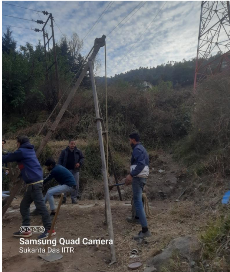
Fig. P7: Dynamic Cone Penetration Test, Near Ropeway Tower No. 1, Manoharbagh (MB1)
