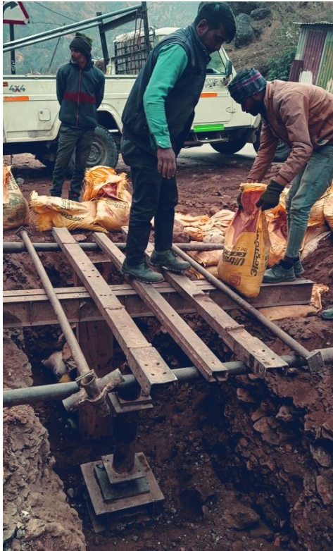
Fig. P1: Field Direct Shear Test at Gandhinagar (GN), Govt. P.G. College (Ward 1)
