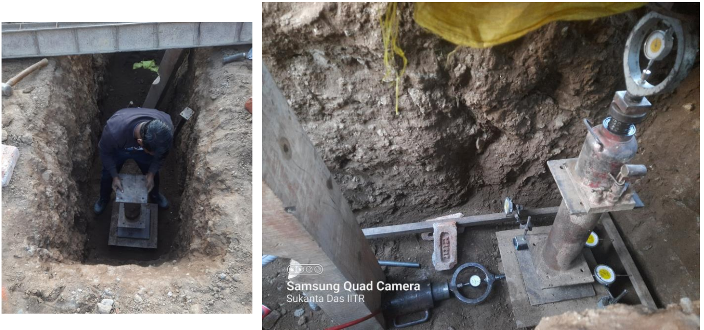
Fig. P9: Field Direct Shear Test, Near PWD Guest House, Manoharbagh (MB2)
