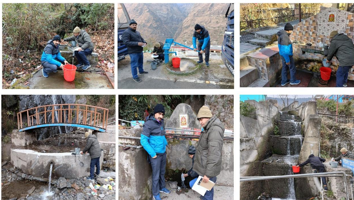
Fig. 13: Survey of various water sources for onsite investigations and collection of samples for laboratory analysis
