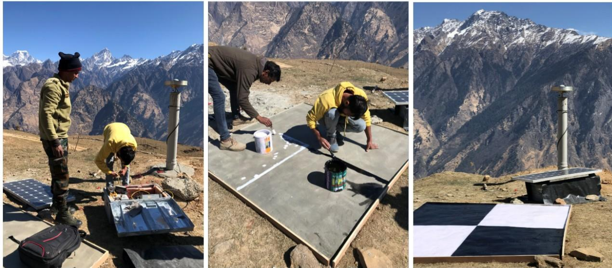
Setting up of Auli GCP & Base Station
