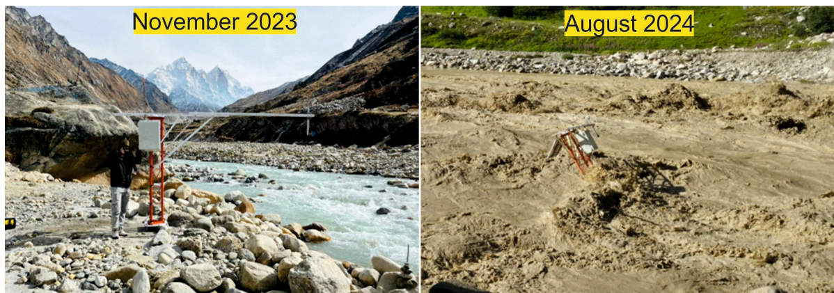
Figure 2: Location of the Automatic Water Level Recorder during the pre-and post-flood events in Bhojwasa.
