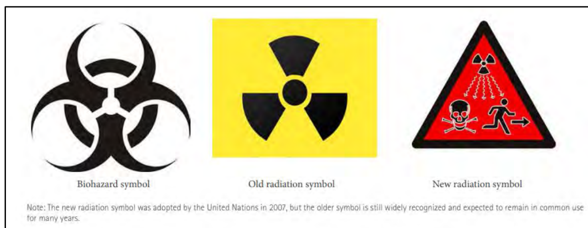
Figure 40: Biohazard, radiation and chemical hazard symbols
