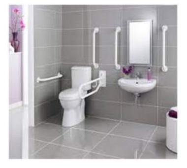
A minimum of one toilet compartment should have enough floor space for a wheelchair user to enter and exit.
