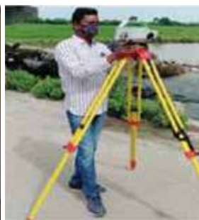
5. Establishment of Ground Control Points
