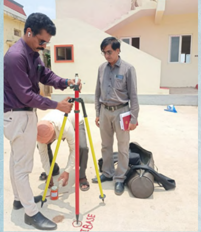
Setting up of Ground Control Points
