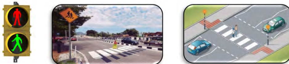
Fig 6.49: Pedestrian crossing signal
