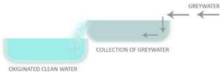
Figure 190 Grey water treatment
