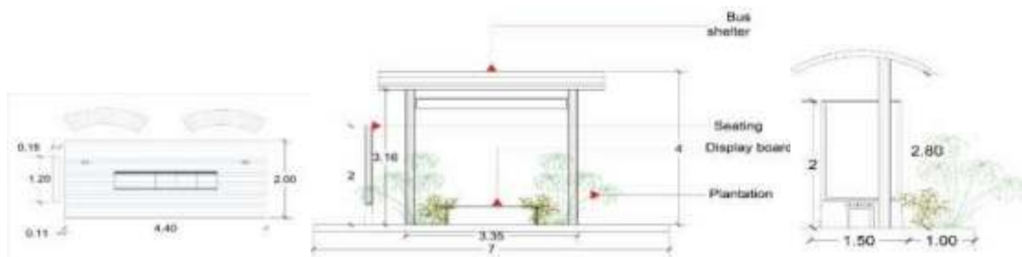
Figure 9-20 Proposed Plan, Section and Elevation for the prototype of bus shelter.
