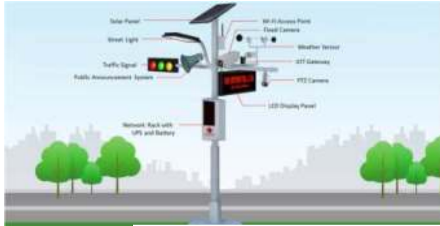
Figure 9-26 Smart utility pole.
