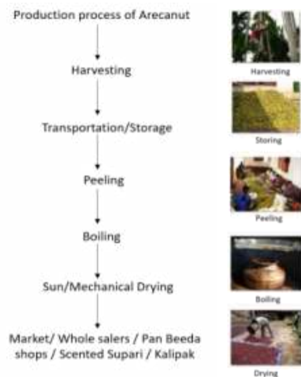
Figure 9-71 Production Process of Arecanut
