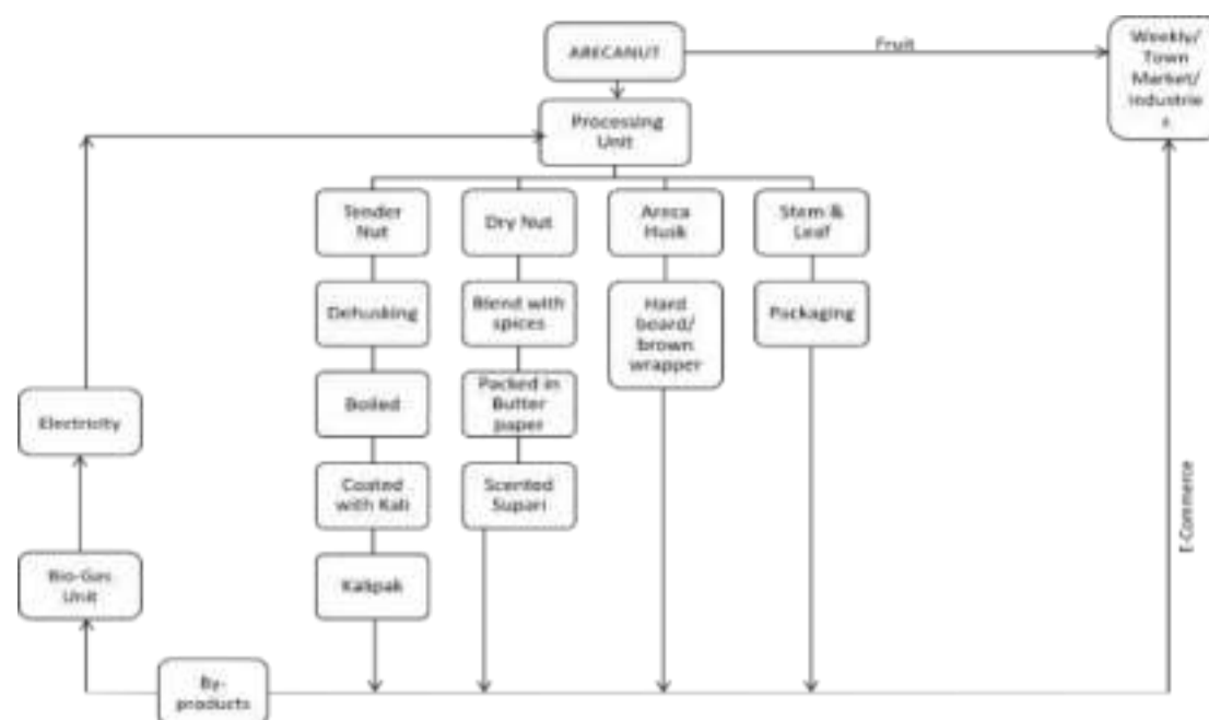
Figure 9-70 Process Flow chart of Arecanut Processing Business in the GP. Source: Author
