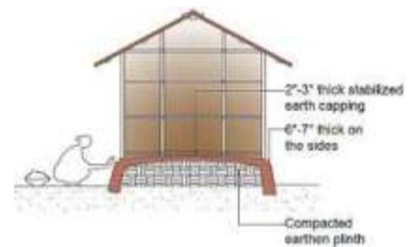
Figure 9-56 Details of cement-stabilized plinth
