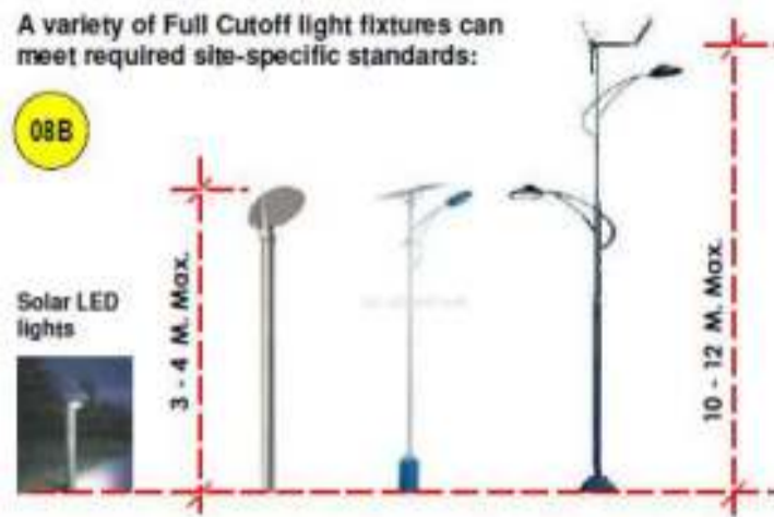
Figure 9-50 Street Light Fixture Detail
