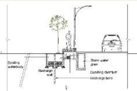
Schematic section showing detail of Recharge well. Source: Author
