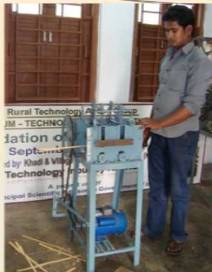
Field trial of slivering machine at Datan, West Medinipur
