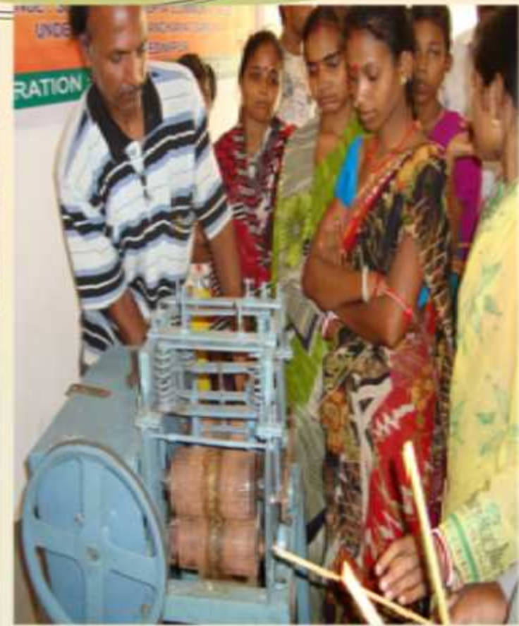
Field trial of slivering machine at Datan, West Medinipur
