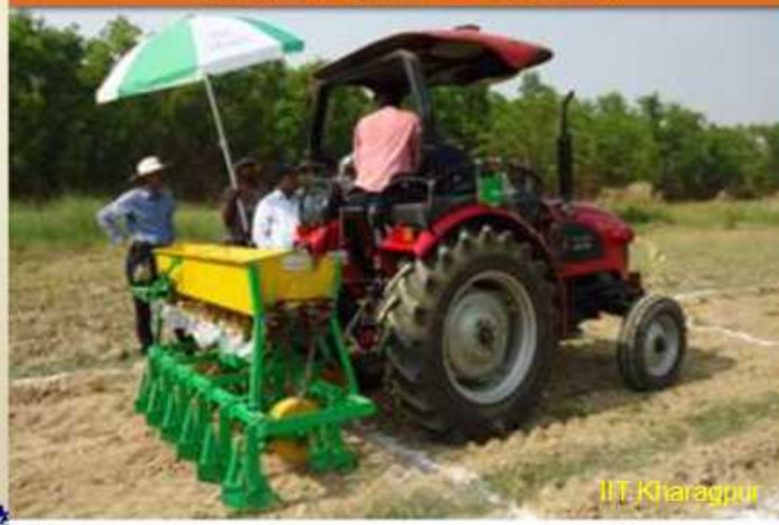
Field Testing of Microcontroller based automatic variable rate fertilizer applicator
