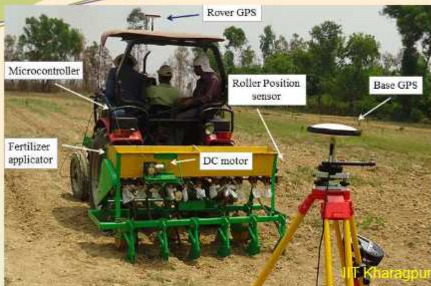
Field Testing of Microcontroller based automatic variable rate fertilizer applicator
