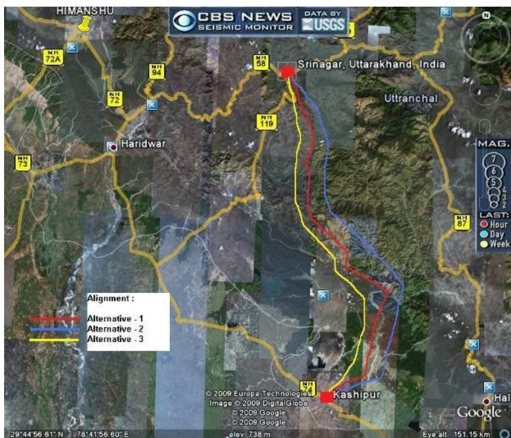
Figure 6: Route Map of 400 kV DC Srinagar - Kashipur transmission line showing the alternatives out of which alternative one is best suitable.
