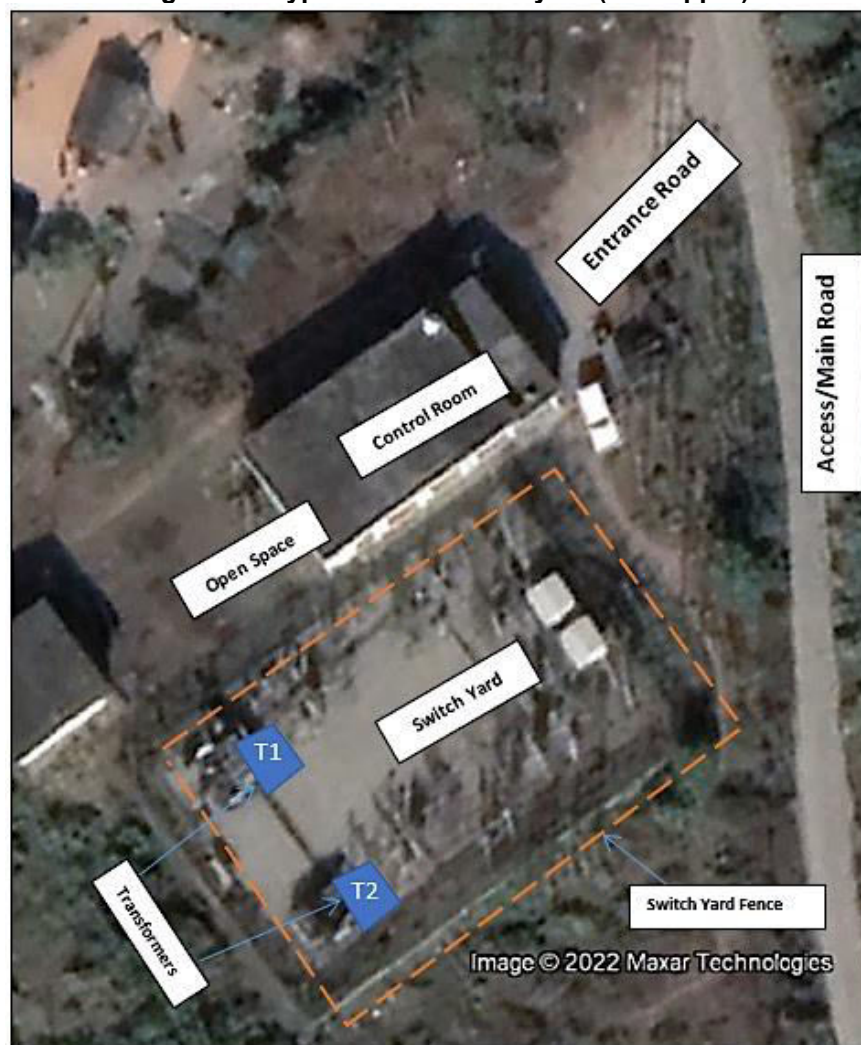
Figure 2.2 Typical substation layout (Lal Tappar)
