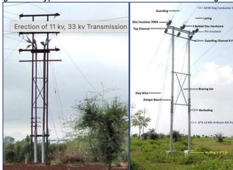
Figure 19: Typical 33/11 kV Poles and Conductor Arrangement
