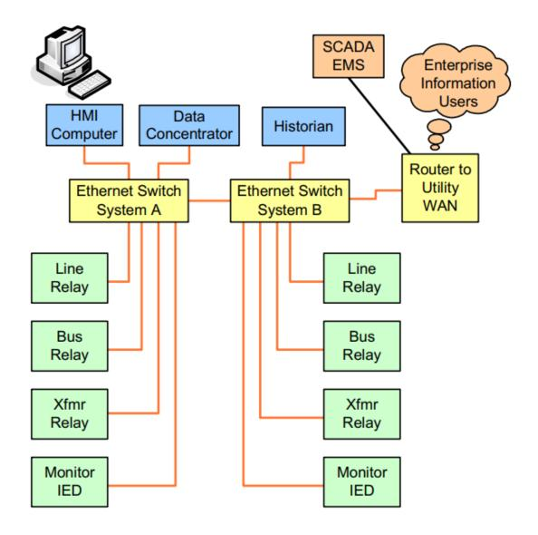
Inter connection of two or more devices with digital communication is the first step towards establishing a network. in addition to the hardware requirements, the software problems of the communication must be solved. Where all the devices on the network are of same make, hardware and software problems are easily solve because the system is design with in same guide lines and specifications.
